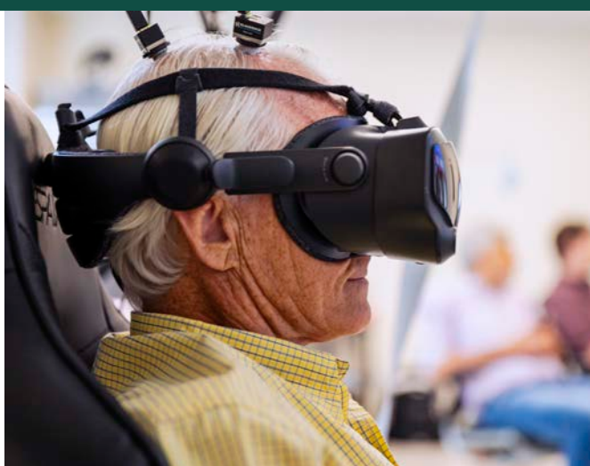
Imbrie wears a virtual reality visor that allows him to see the virtual arm he is trying to manipulate using signals sent through the electrodes in his brain.
